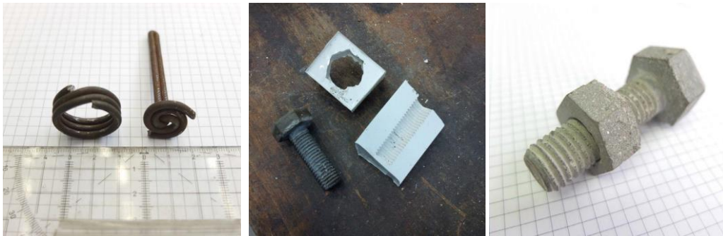
Figure 1: The concrete screws for the canoe: reinforcement (left), formwork (middle) and completed concrete screw with nut (right)
